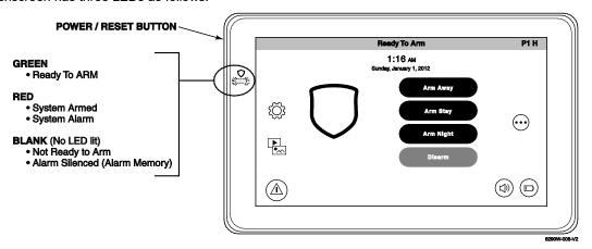
To reset the Touchscreen, press and hold the side **Power Button** for 3 seconds and **t**hen select the reset button **O** on the screen to start the reset function. The Touchscreen can also be reset by pressing and holding the reset button for approximately15 seconds until the touchscreen resets automatically.
